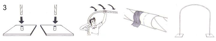
Place the tubes in the foot parts and press down firmly.
