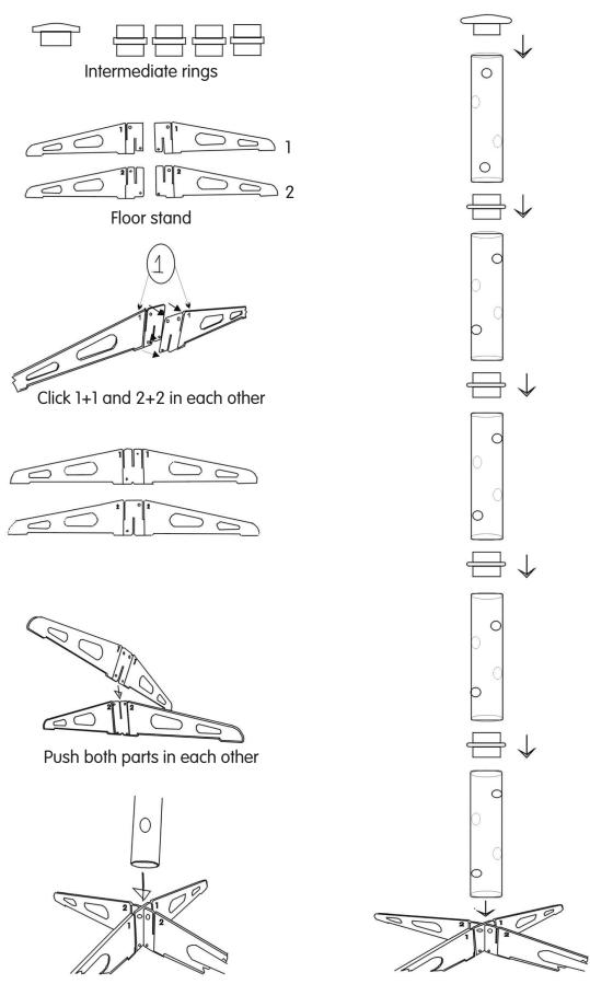
Put the tubes with the intermediate rings in the floor stand
