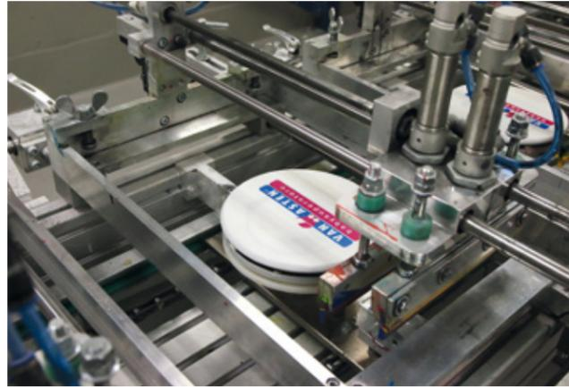
For accurate multi-colour motifs, the balloons are pulled onto a plate prior to being imprinted.
